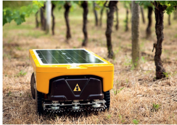
The Vitirover is only 70 centimeters long and weighs slightly under 20 kilograms. It cuts grass and weeds at a rate of 300 meters per hour.
